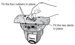
4. Fix the Ceiling Plate A to the Ceiling Plate B and fix them firmly with Screws A.
